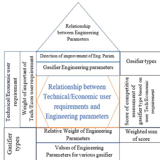
Fig. 2 Schematic of QFD/MCDM Framework
