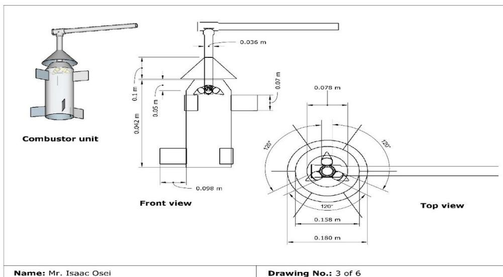
**Fig. 12 Schematic Diagram of the Combustor and Nozzle Assembly**
