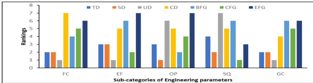
**Fig. 4 Ranking of the Various Gasifier Types Under the Various Technical Sub-Categories Parameters**
