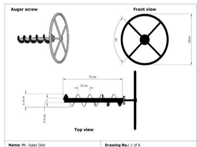
**Fig. 10 Schematic Diagram of Gasifier Screw Auger System**
