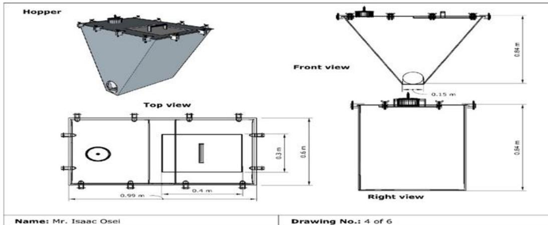
**Fig. 8: Schematic Diagram of Gasifier Hopper Assembly**
