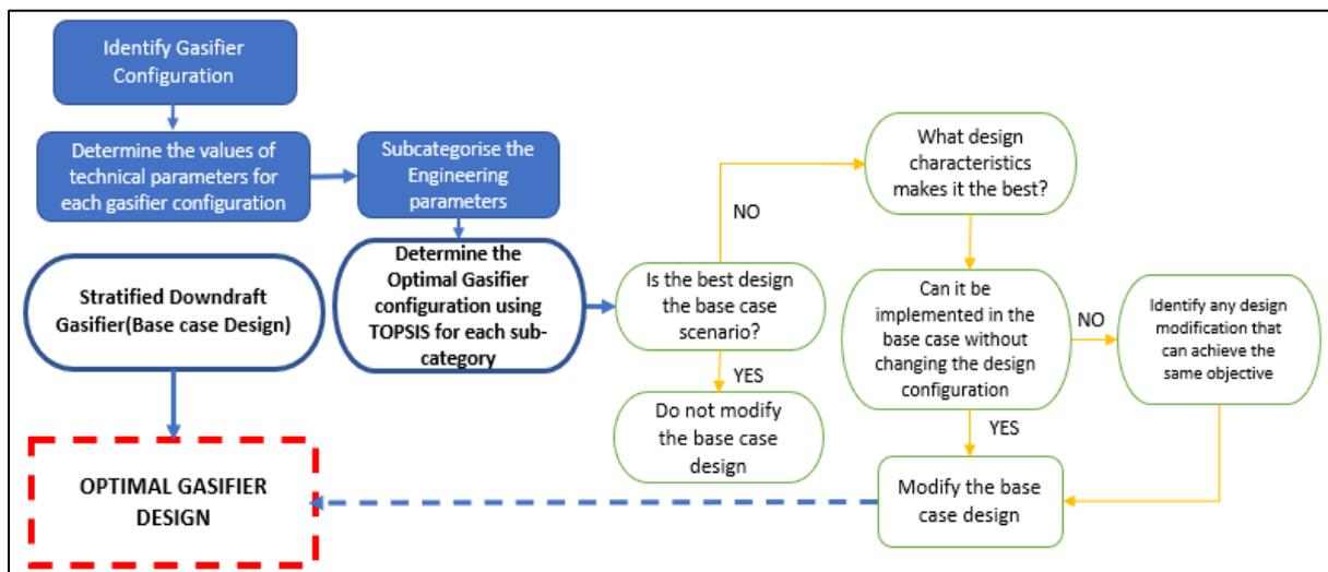
Fig. 3 Schematic for the Design of the Gasifier Reactor
