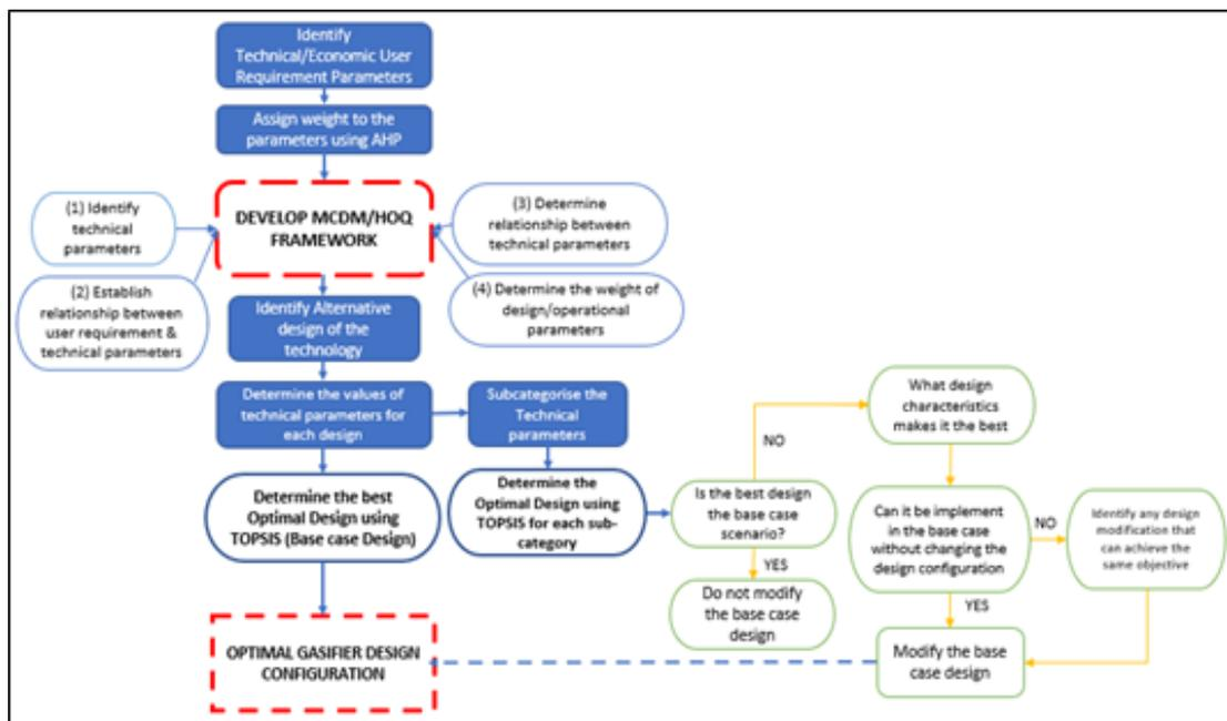
Fig. 1 MCDM/QFD Model for Design of Optimal Gasifier
