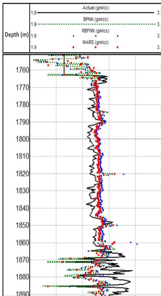
**Fig. 4 Prediction Performance of Density Log Response for MARS, BPNN and RBFNN**
