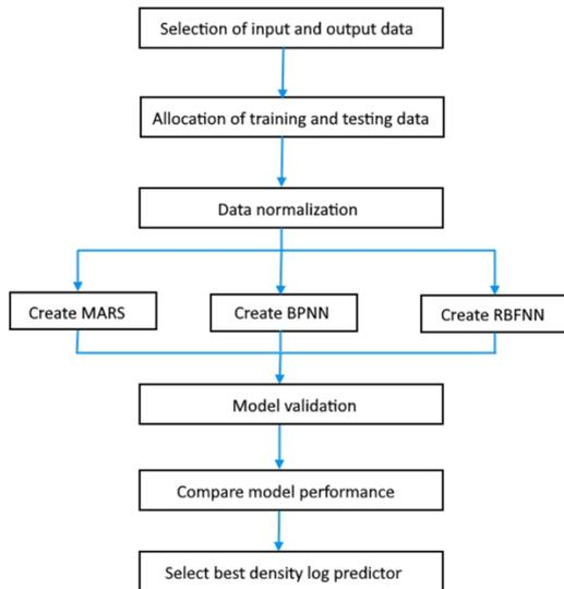
**Fig. 3 Workflow of Developing MARS, BPNN and RBFNN for Density Log Prediction**
