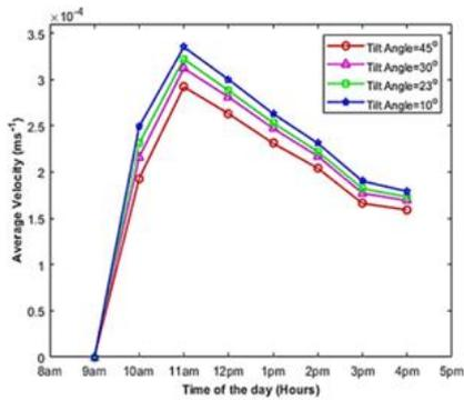
**Fig. 8 Effect of Tilt Angle on Average Velocity Distribution in the Collector Tube**
