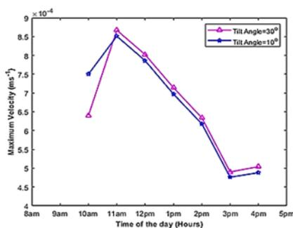
**Fig. 9 Effect of Tilt Angle on Maximum Velocity in the Collector Tube**
