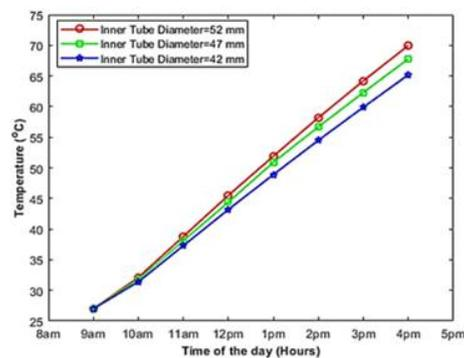
**Fig. 5 Effect of Collector Diameter on Temperature Distribution in the Storage Tank**
