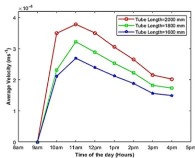
**Fig. 6 Effect of Collector Length on Velocity Distribution**
