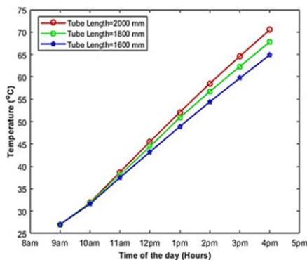
**Fig. 4 Effect of Collector Length on Temperature Distribution in the Storage Tank**
