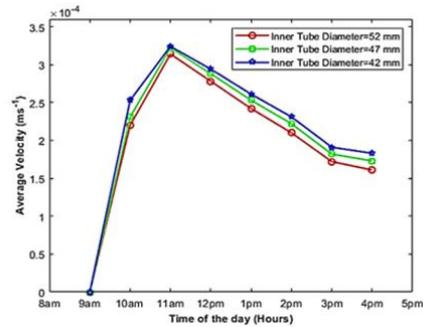
**Fig. 7 Effect of Collector Diameter on Velocity Distribution**
