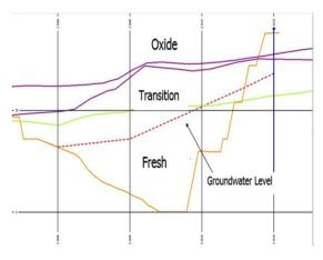
Fig. 3 Schematic Hydrogeological Model showing the Phreatic Water Surface
