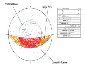
Fig. 5 Wedges Sliding Potential Analysis for the East Wall
