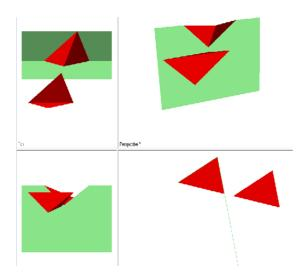
Fig. 6 Determination of Volume of Wedges using "SWEDGE"
