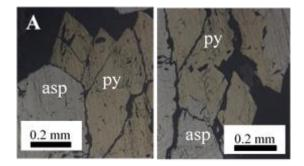
Fig. 4 Photomicrograph (A and B) Showing Mutual Boundary Textures between Pyrite and Arsenopyrite
