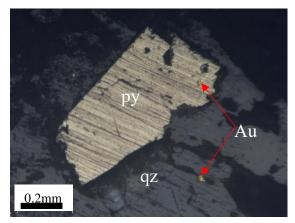
Fig. 7 Photomicrograph Showing Gold in Quartz (Free-milling Ore) and as an Inclusion in Pyrite (Refractory Ore)
