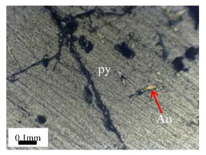
Fig. 6 Photomicrograph showing gold occurring as Inclusion in Pyrite
