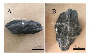
Fig. 2 Photographs (A) and (B) Showing Samples from the Transition Zone
