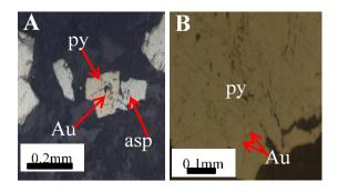
Fig. 5 Photomicrograph (A and B) Showing Gold Occurrence as (A) Cavity-fill in Pyrite (Free-milling Ore) and (B) Inclusion in Pyrite (Refractory Ore)
