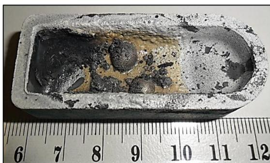
**Fig. 11** Droplets of Metallic Iron obtained after Reduction of Fe<sub>2</sub>O<sub>3</sub>-PC Composite at 1250 °C
