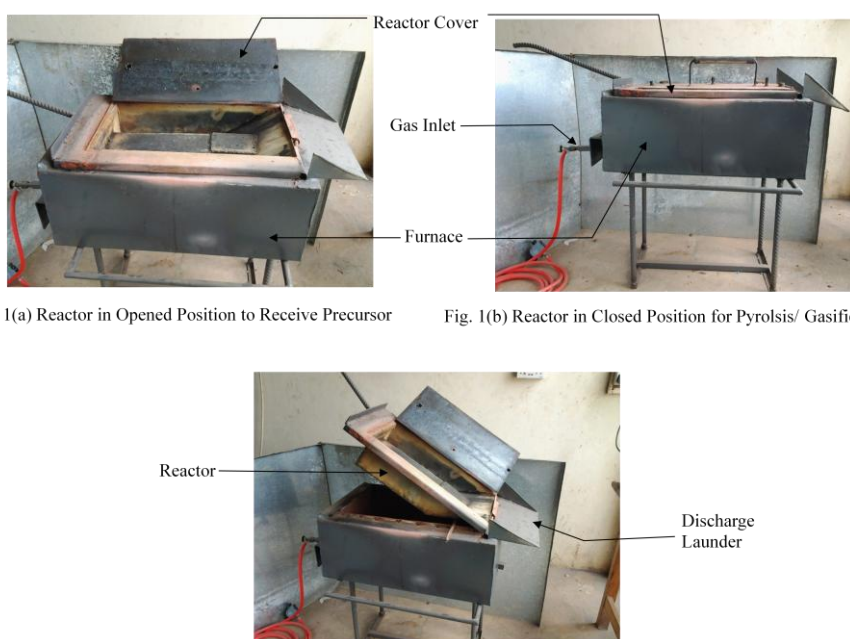
Fig. 1(c) Reactor Lifted for Discharging of Carbonaceous Products
