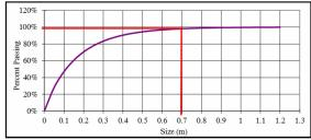
Fig. 9 Kuz-Ram Model for Mine Blast
