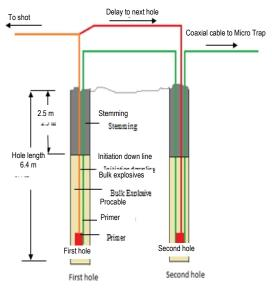
Fig. 2 Setup for VOD Measurement
