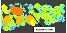
Fig. 11 Delineated Photo of Muckpile
