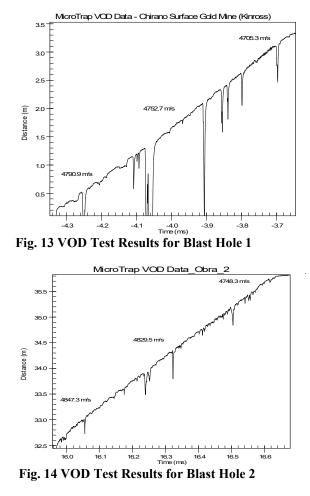
From Figs. 13 and 14, the average VOD values of the blend emulsion explosives are 4 759.6 m/s and 4 808.4 m/s for blast hole 1 and blast hole 2 respectively. These average values were slightly above (1.3% and 2.3%) the manufacturer's theoretical VOD value of 4 700 m/s for Emunex 7000 (70% Emulsion, 30% ANPP). This indicates that the performances of the explosive accessories and the bulk explosives were very good.
