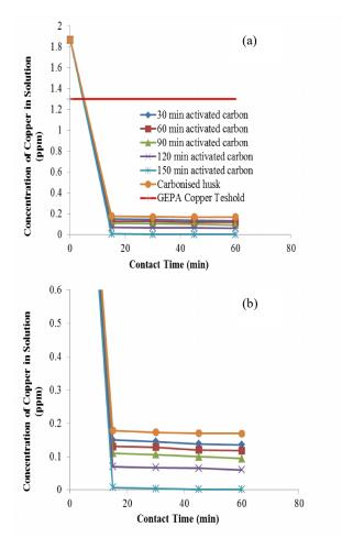
Fig. 4 Concentration Profile of Copper in the Wastewater in Relation to Adsorption Time: (a) For 0 to 1.87 ppm of Copper Concentration (b) For 0 to 0.60 ppm of Copper Concentration
