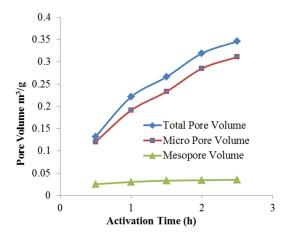
Fig. 3 Pore Volumes of the Activated Carbons Relative to Activation Time
