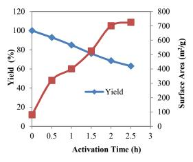
Fig 2 Yield of Activated Carbons Relative to Activation Time
