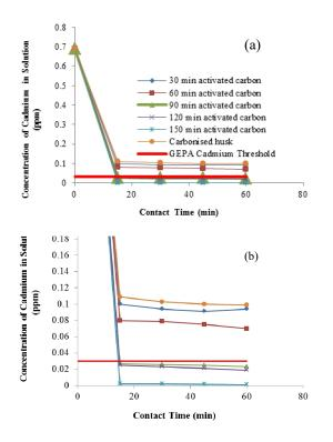
Fig. 5 Concentration Profile of Cadmium in the Wastewater in Relation to Adsorption Time: (a) For 0 to 0.69 ppm of Cadmium Concentration (b) For 0 to 0.18 ppm of Cadmium Concentration
