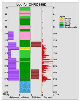
Fig. 15 Graphic Log of Drill Core showing Structural Matrix at Akwaaba
