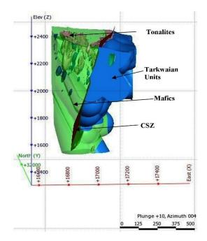
Fig. 13 Leapfrog Model of Akwaaba Deposit illustrating Geology and Shear
