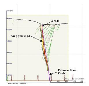
Fig. 9 North Section of Paboase Deposit showing the Various Structural Shapes
