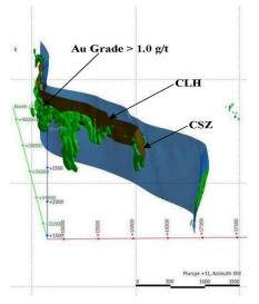
Fig. 16 A 3-D Model of Chirano Structures and Gold Grade on a District Scale
