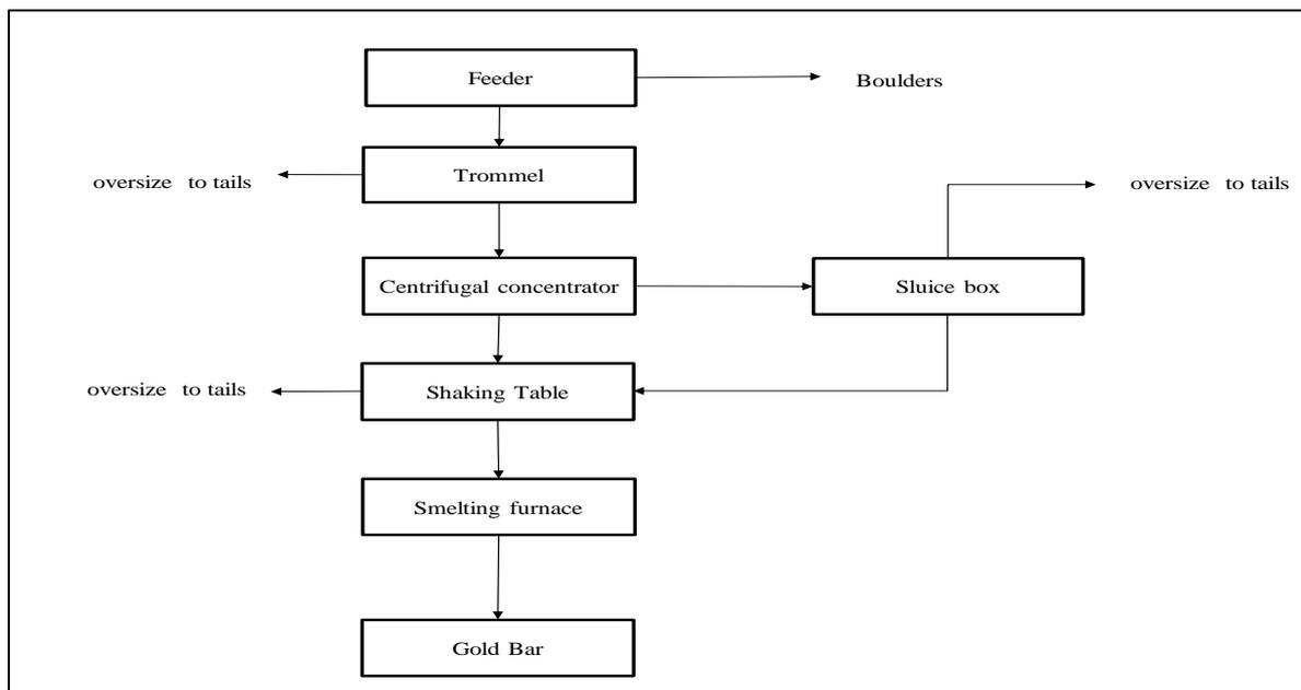
**Fig. 6 Alluvial Deposit Proposed Flow Sheet**
