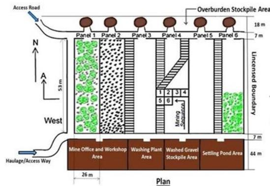
**Fig. 4 Strip Mining Method (Source: Mireku-Gyimah and Tsidzi, 1996)**
