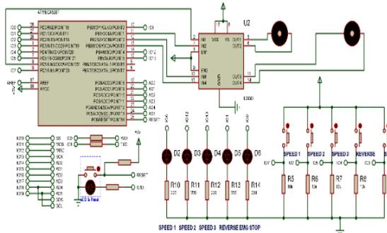
**Fig. 3** Proteus Simulation Model for Speed of the Conveyor System
