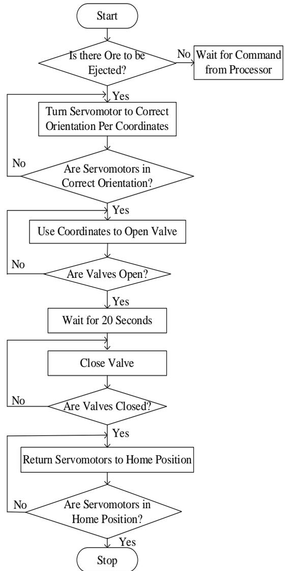
**Fig. 2 Flowchart of the Separation Mechanism**
