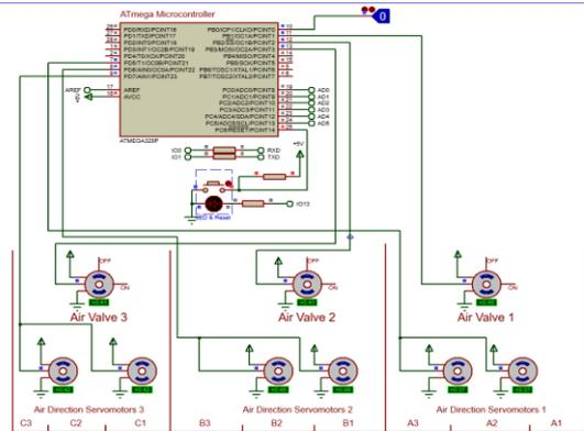
**Fig. 4** Proteus Simulation Model for the Separation Mechanism
