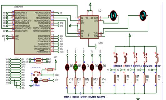
**Fig. 6** Conveyor System Operating at Speed 2 of Value 3.2 m/s
