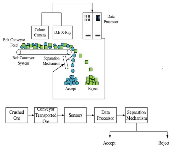
**Fig. 1 Functional Diagram of the Proposed Design of Sensor-based Ore Sorting**
