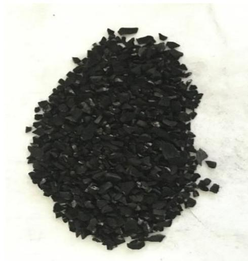
**Fig. 2 Locally Prepared Activated Carbon (CS-AC)**
