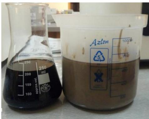
**Fig. 3 Drilling Mud Separated into the Solid and Liquid Phases**
