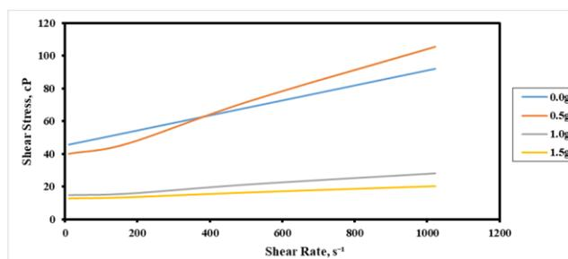
**Fig. 4 Rheogram of Equilibrium Zeolite WBM Sample at 120 °F**
