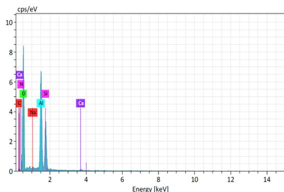
**Fig. 2 Energy-Dispersive X-Ray Spectroscopy Plot for Equilibrium Zeolite**
