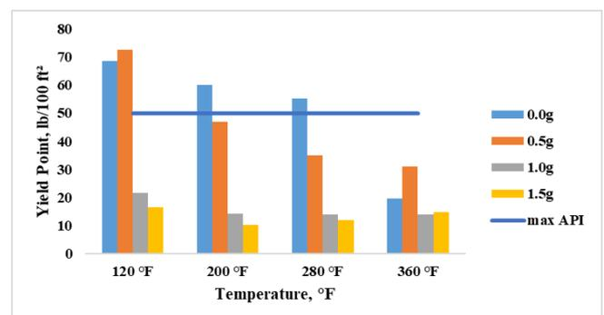
Fig. 9 Yield Point of Equilibrium Zeolite Base Mud Sample at Varying Temperatures
