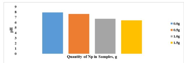
**Fig. 14 pH of Varying Quantities of Equilibrium Zeolite in Mud Samples**
