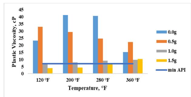
Fig. 8 Plastic Viscosity of Equilibrium Zeolite Base Mud Sample at Varying Temperatures
