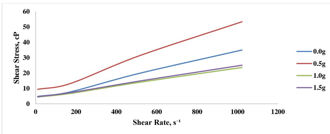
Fig. 7 Rheogram of Equilibrium Zeolite WBM Sample at 360 °F
