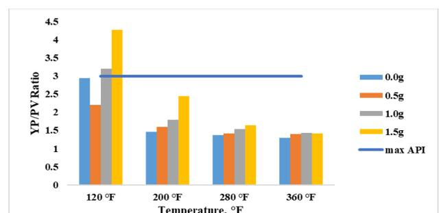
Fig. 10 YP/PV Ratio of Equilibrium Zeolite Base Mud Sample at Varying Temperatures
