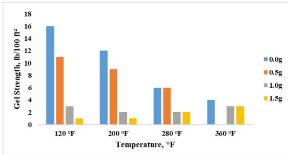
**Fig. 11 Ten Seconds Gel Strength of Equilibrium Zeolite Base Mud Sample at Varying Temperatures**
