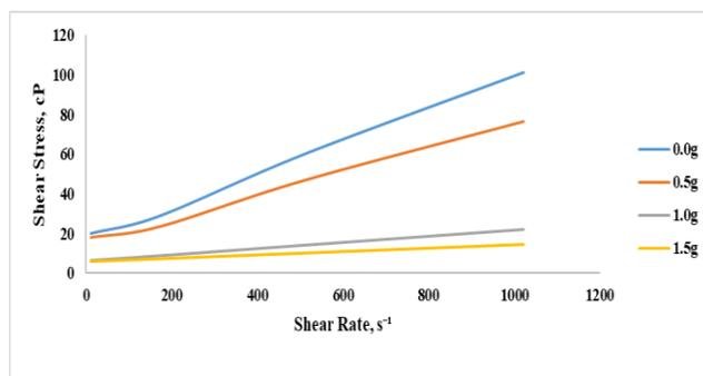
**Fig. 5 Rheogram of Equilibrium Zeolite WBM Sample at 200 °F**
