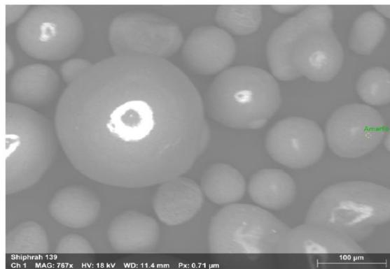
**Fig. 3 Equilibrium Zeolite Scanning Electron Microscope Image**
