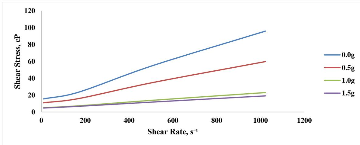
Fig. 6 Rheogram of Equilibrium Zeolite WBM Sample at 280 °F
