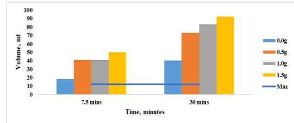
**Fig. 13 Filtration Loss of Equilibrium Zeolite Base Mud after 7.5 and 30 Minutes**
