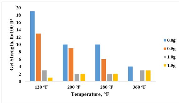
**Fig. 12 Ten Minutes Gel Strength of Equilibrium Zeolite Base Mud Sample at Varying Temperatures**
