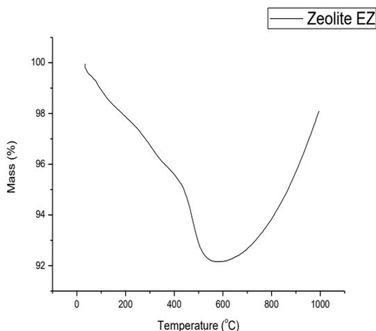
**Fig. 1 Thermogravimetric Analysis Chart for Equilibrium Zeolite**
