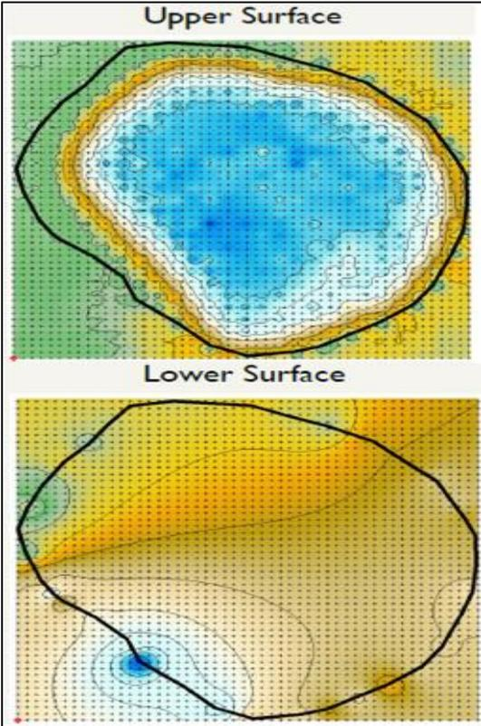
**Fig. 11 Upper and Lower Surface of Stockpile C**
