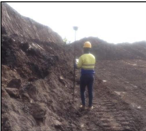
**Fig. 4 Picking Crest and Toe with GPS Receiver**
