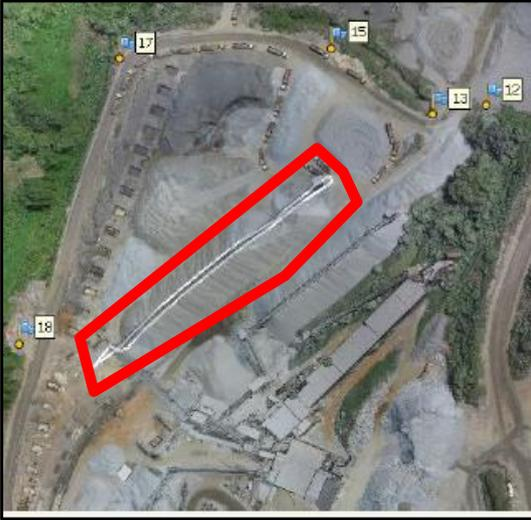
**Fig. 12 Orthophoto of Stockpile D with Conveyor Belt**
