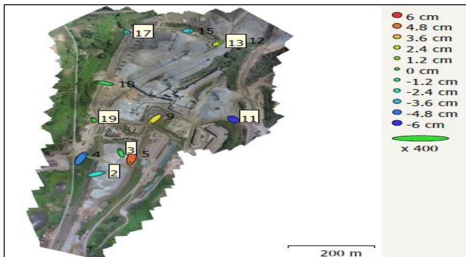
**Fig. 7 Orthophotos with Ground Control and Check Points**
