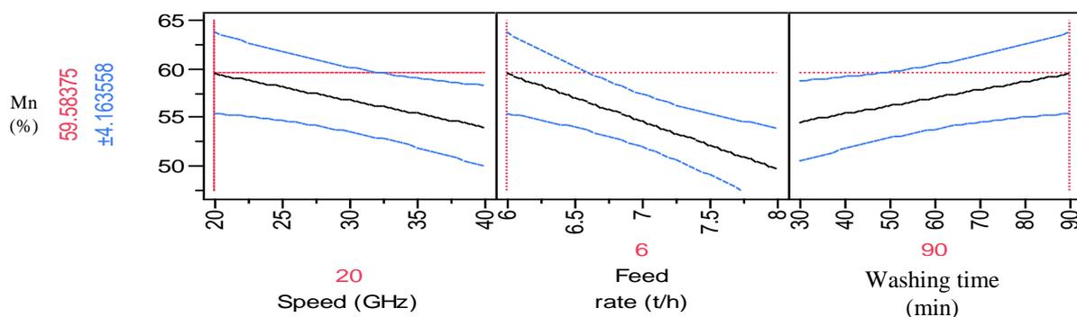
**Fig. 3 Prediction profile for Mn grade (%) as A Function of Speed, Feed Rate and Washing Time**
