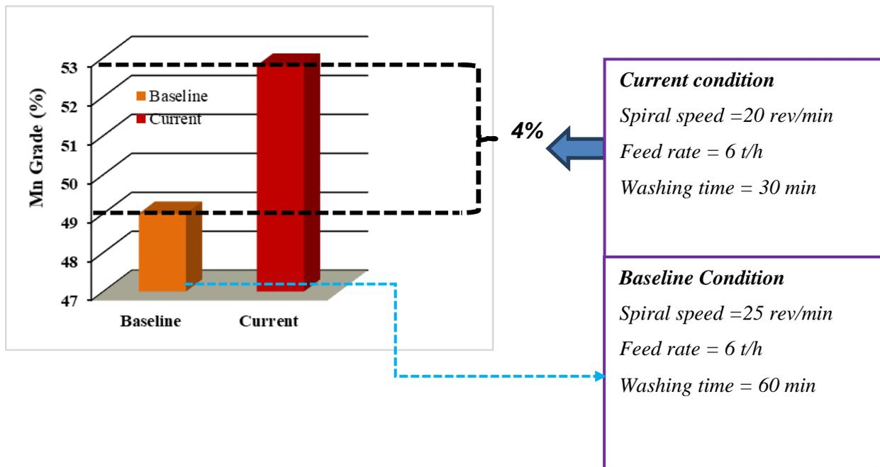
Fig. 5 Mn Grade (%) as a Function of Plant Condition and Simulated Condition
