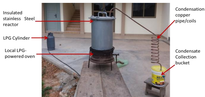
Fig. 3 Locally, Fabricated LPG-Powered Pyrolysis Process Setup
