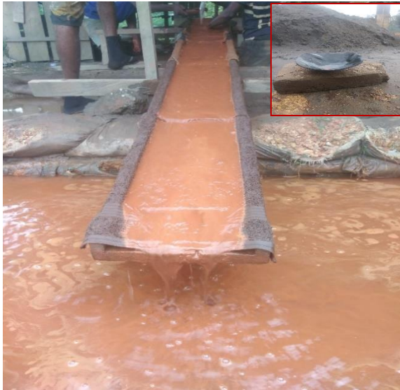
Fig. 1 Sluicing and Panning Operations of ASGM
