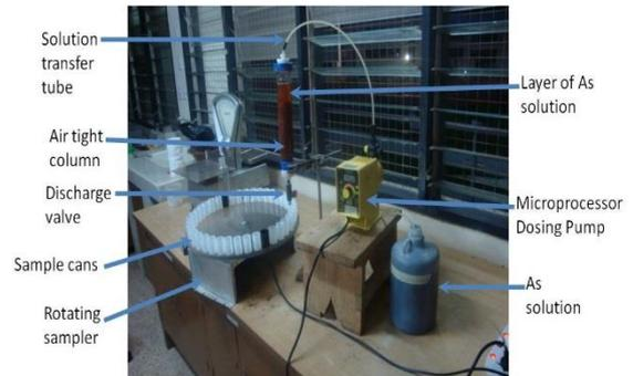
**Fig. 1 Experimental Set Up for Sorption and Desorption Test Work**
