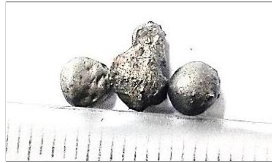
Fig. 18 Metallic Iron Nuggets formed from Slag Sample after Firing
