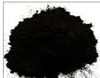
Fig. 3 Samples of Pulverised Charred Electrical Socket
