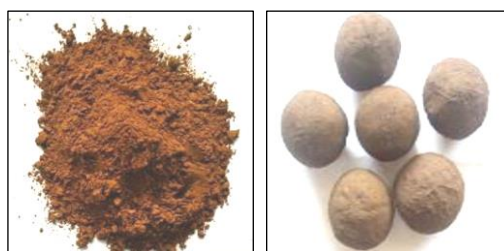
Fig. 4 Spherical Pellets formed from Milled Ore Sample and WES
