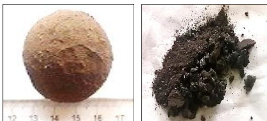
Fig. 17 Green Ore Pellet before and after Firing Slag-WES Composite Pellet
