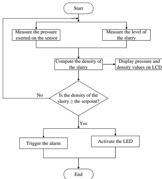
**Fig. 3 Flowchart for the Slurry Anti-Hardening System**
