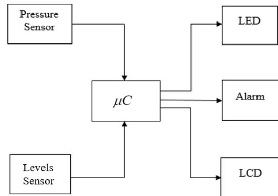
**Fig. 2 Block Diagram of the Integrated Anti-Hardening System**
