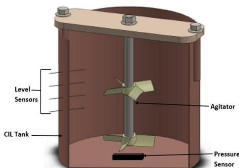
**Fig. 1 Design Concept Representation of Slurry Anti-Hardening System**
