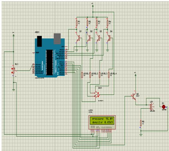
**Fig. 6 Screenshot of Simulation of Designed Circuit (Red LED and Buzzer ON)**
