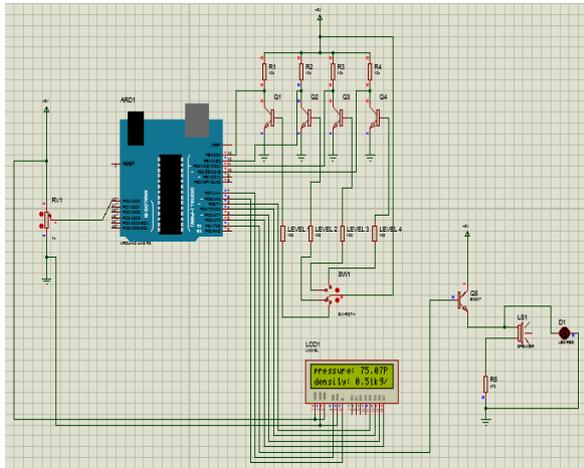
**Fig. 5 Screenshot of Simulation of Designed Circuit (Red LED and Buzzer OFF)**
