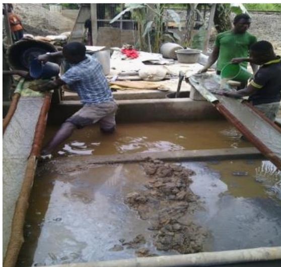
**Fig. 1 Gravity Concentration by Sluicing**
