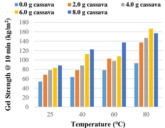
**Fig. 4 Ten Minutes Gel Strength of Cassava Starch Mud Formulations vs. Temperature**
