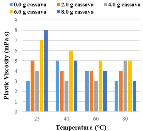
**Fig. 1 Plastic Viscosity of Cassava Starch Mud Formulations at Different Temperature**
