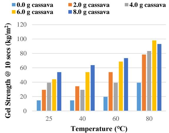
**Fig. 3 Ten seconds Gel Strength of Cassava Starch Mud Formulations vs. Temperature**
