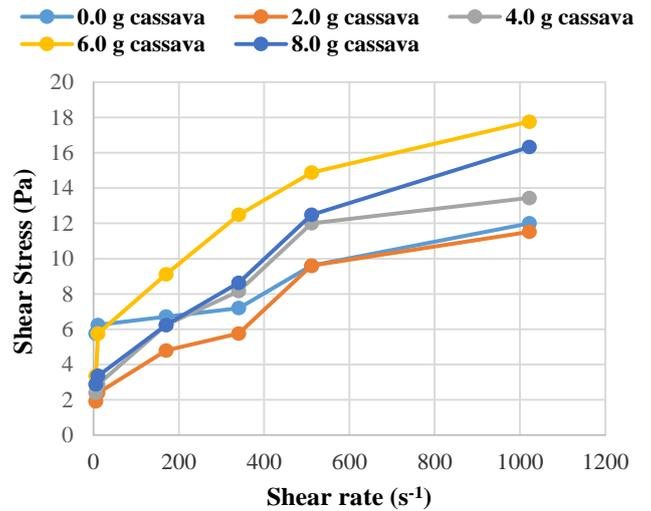
Fig. 7 Rheogram showing Fluid Behaviour at 40 °C
