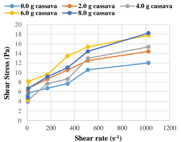
Fig. 9 Rheogram showing Fluid Behaviour at 80 °C
