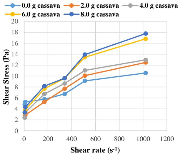
Fig. 6 Rheogram showing Fluid Behaviour at 25 °C
