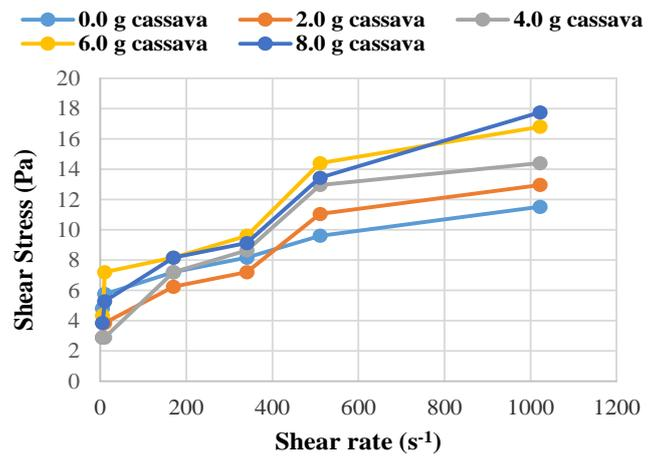
Fig. 8 Rheogram showing Fluid Behaviour at 60 °C
