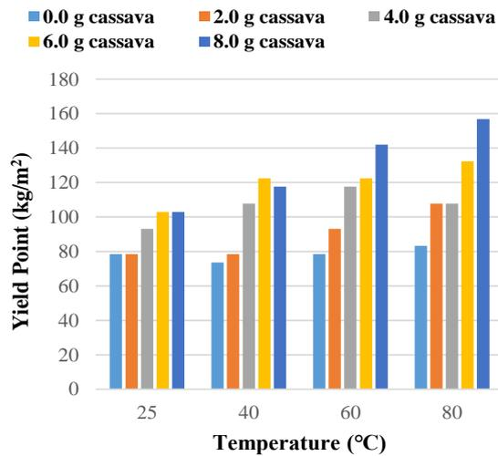
**Fig. 2 Yield Point of Cassava Starch Mud Formulations vs. Temperature**
