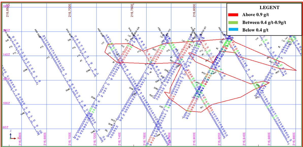
Fig. 1c Section at 1532600 N showing Digitised Ore Zone
