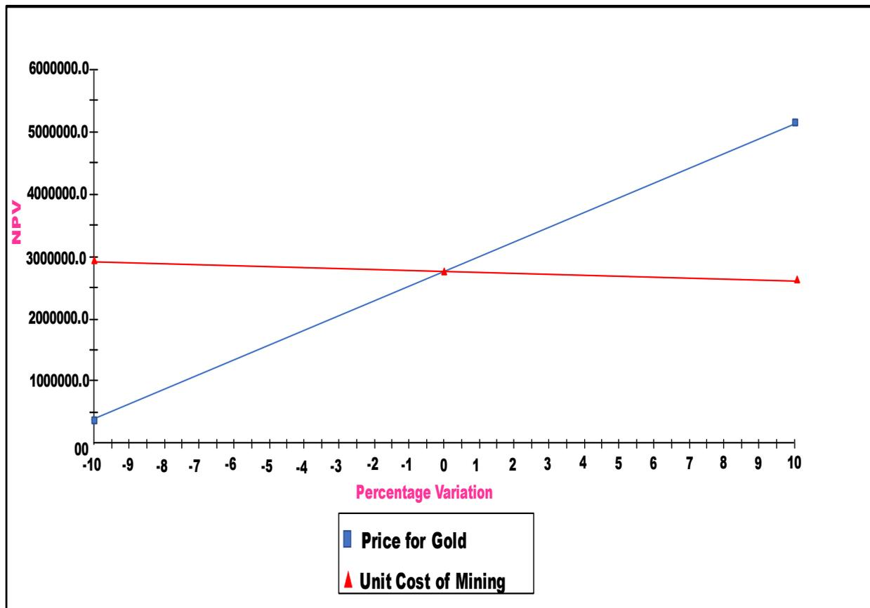
**Fig. 7 Sensitivity of Discounted Cashflow (NPV) to Various Parameters**
