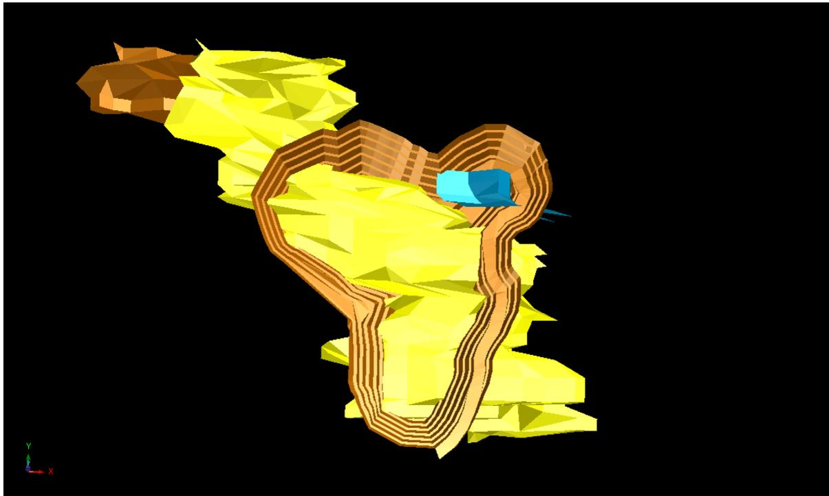
**Fig. 11 Detail Pit Design Superimposed on the Solid Model**
