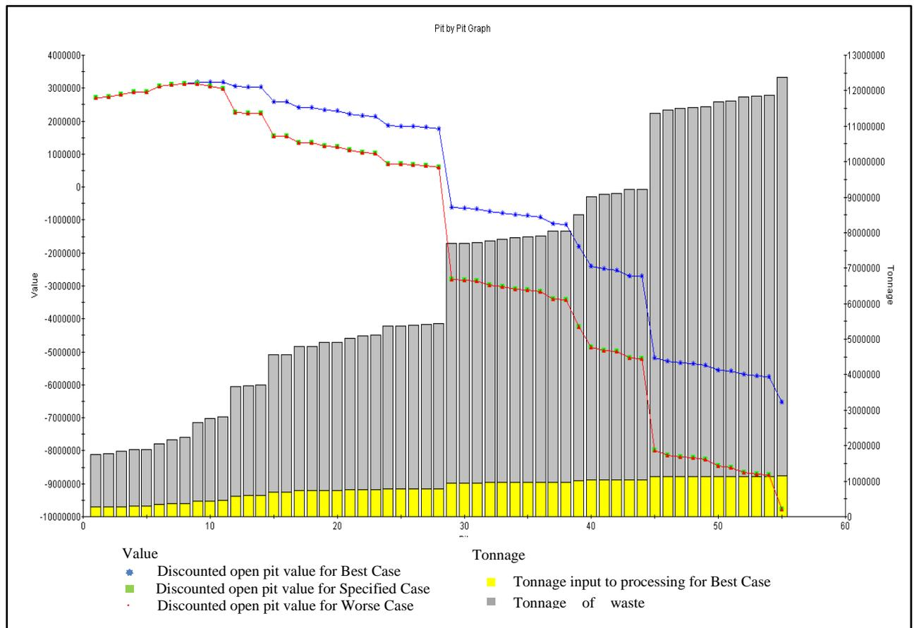
**Fig. 6 Total Ore and Waste Tonnage versus NPV Value of Nested Pit**
