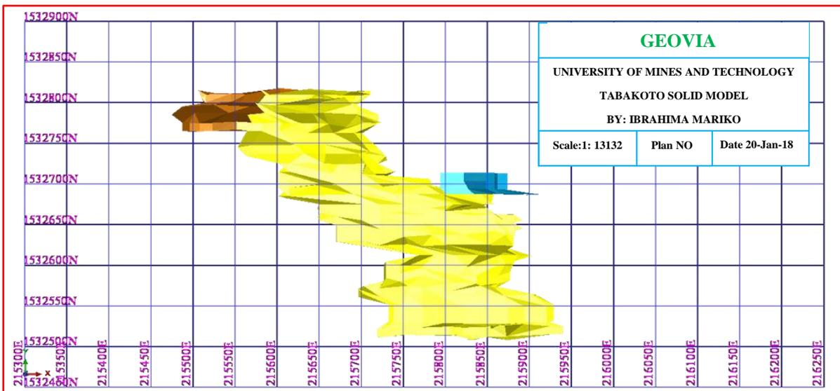
Fig. 2 Solid Model of the Tabakoto Deposit
