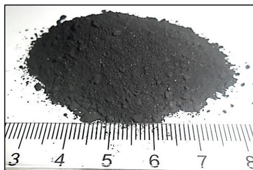
Fig. 3 Pulverised Mass obtained from Spent TigerHead Battery
