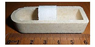
Fig. 5 Cylindrical Pellet of Nsuta Rhodochrosite Ore in a LECO<sup>TM</sup> Crucible
