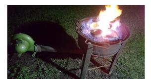
Fig. 3 Firing of Crucibles containing Samples
