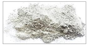
Fig. 1 Pulverised Nsuta Rhodochrosite
