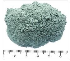
Fig. 3 Samples of Pulverised Carbonaceous Material obtained from Heat-treated HDPE
