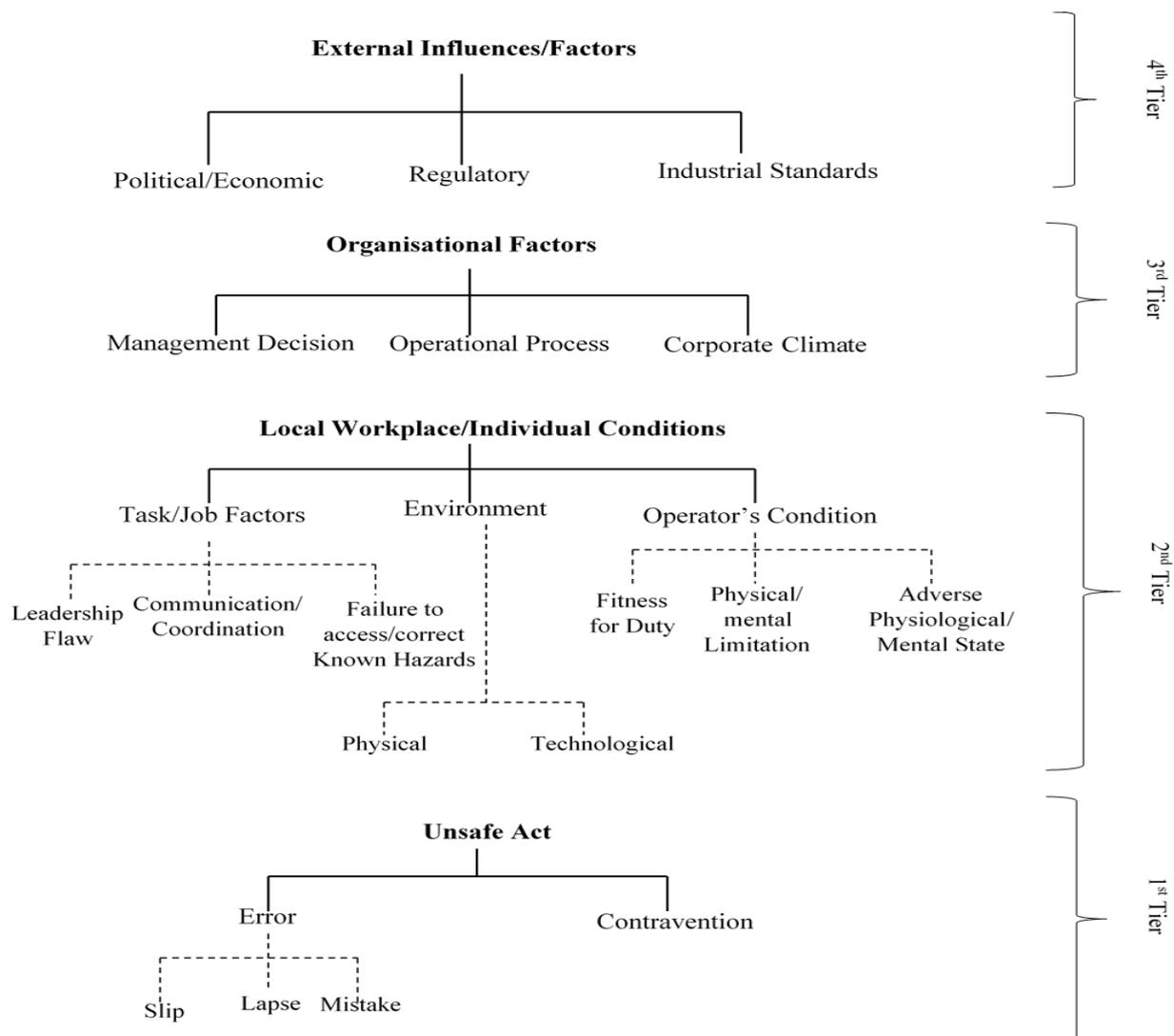
**Fig. 9 Human Factor Analysis and Classification System-Ghana Mining Industry (HFACS-GMI) Framework**
