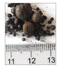
Fig. 15 Samples of Reduced Metal obtained after Reduction at 1550 °C
