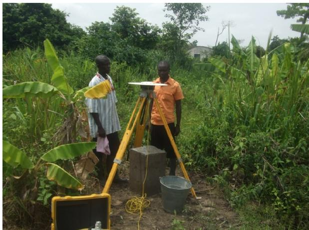
**Fig. 6 GPS Observation Over a Pillar along the Boundary**
