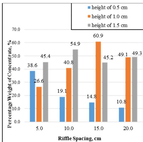
**Fig. 7 Percentage Weight of Concentrate at Various Riffle Heights and Spacing**
