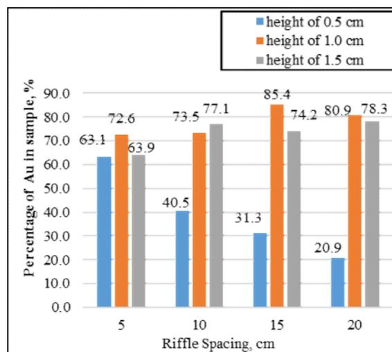
**Fig. 8 Percentage of Gold in Concentrate Obtained at Various Riffle Heights and Spacing**
