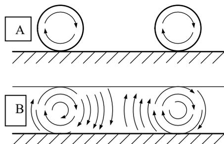
**Fig. 1 (a) Movement of Spherical Solid Particles and (b) Turbulent Whirl Flow**
