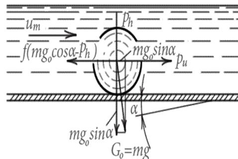
**Fig.3 Forces Acting on a Body in the Water Stream Flowing on an Inclined Plane**
