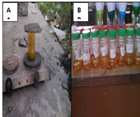
Fig. 6 Digestion of Sample (A) and Labelled Containers with Filtrate Ready for AAS Analysis (B)
