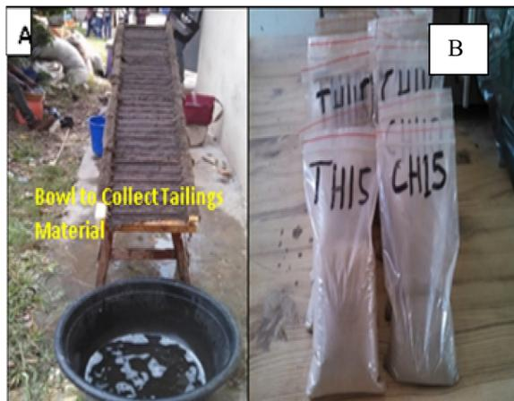
Fig. 5 (A) Sluicing Set-Up and (B) Labelled Samples of Concentrate and Tailings
