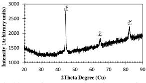
Fig. 16 XRD of Reduced Mass showing Peaks of Metallic Iron
