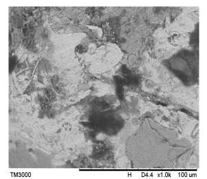
Fig. 12 SEM Photomicrograph of Reduced Agbaja Iron Ore
