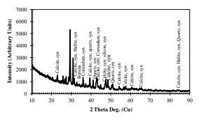
Fig. 7 XRD Patterns of Ash obtained after the Charring Process
