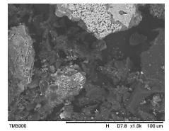
Fig. 6 SEM Photomicrograph of Ash obtained after Charring of WES
