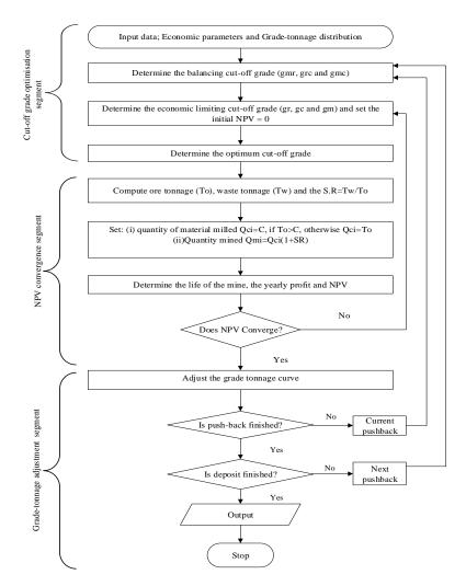
Fig. 3 Logic Flow Diagram of the Lane's Approach (After Bascetin and Nieto, 2007)
