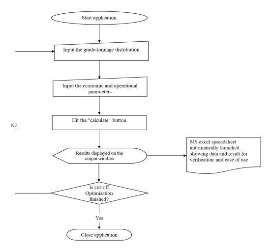
Fig. 4 Process Flowchart of the Working of Cut-Off Optimiser Ver.1.0
