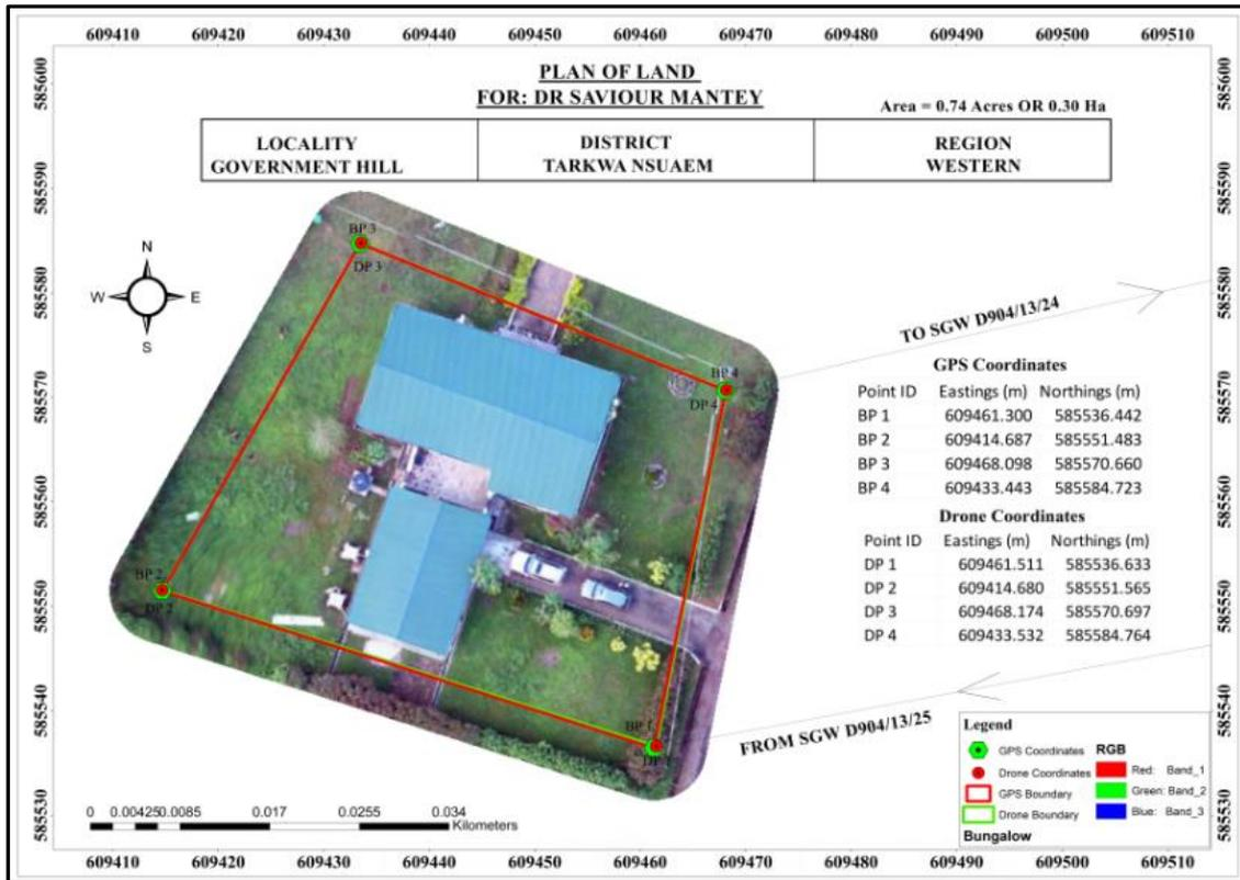
**Fig. 8 Overlay of GNSS and UAV Cadastral Plans on Orthophoto of Study Area**
