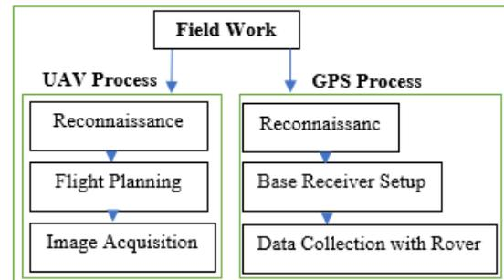
Fig. 4 UAV and GNSS Survey Fieldwork Procedure
