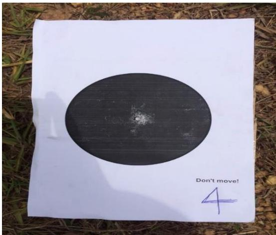
Fig. 2 Ground Control Point (Target)
