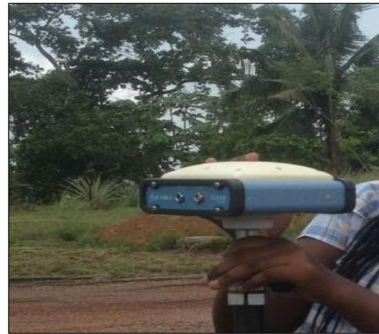
Fig. 3 South S86 GNSS Receiver
