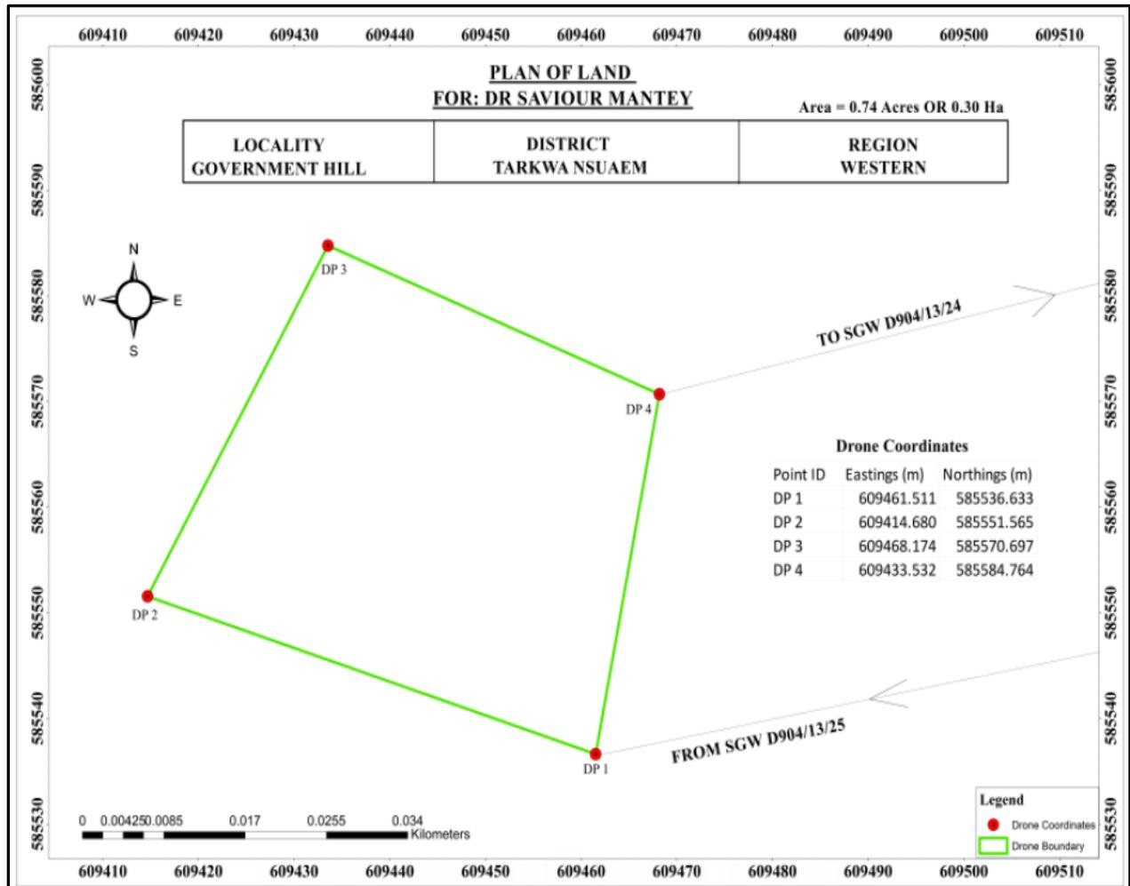
Fig. 5 Cadastral Plan from UAV Surveys
