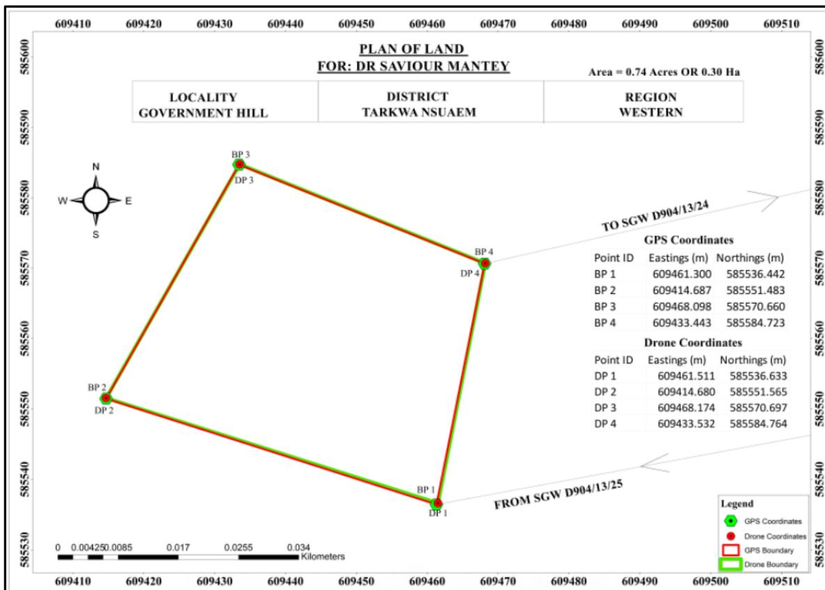
Fig. 7 Overlay of Cadastral Plan from UAV and GNSS Surveys
