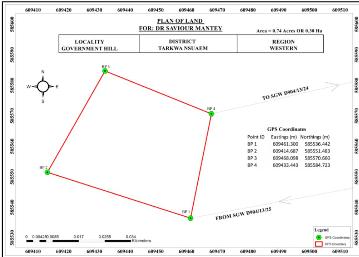
Fig. 6 Cadastral Plan from GNSS Surveys
