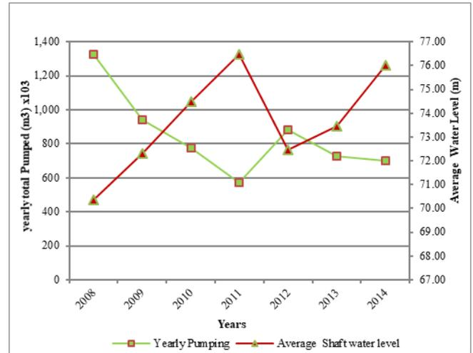
Fig.9 Average Groundwater Elevations vs. Yearly total Pumped (2008-2014).
