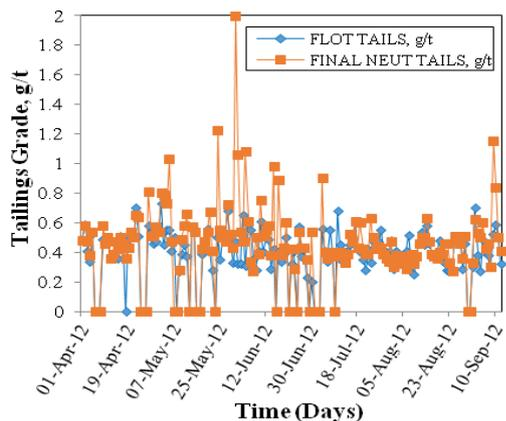
**Fig. 8 Comparison of Gold Grades of Neutralisation and Flotation Tailings**
