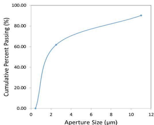
Fig. 1 PSD of suspended particles in the CCDO
