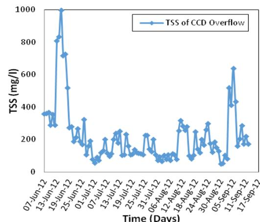
**Fig. 7 TSS of CCDO after Introducing QT**
